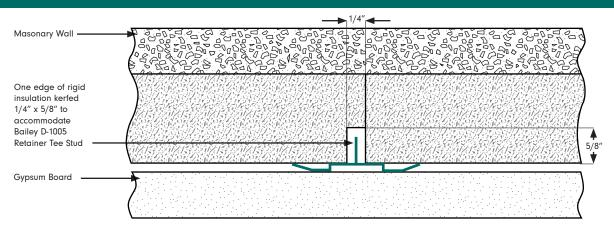
**NOTE:** The Retainer Tee can be installed with square edged or ship tap panels with or without the field kerf being applied. In the completed installation, the back of the gypsum board is tight to the face of the insulation (no air space exists).
